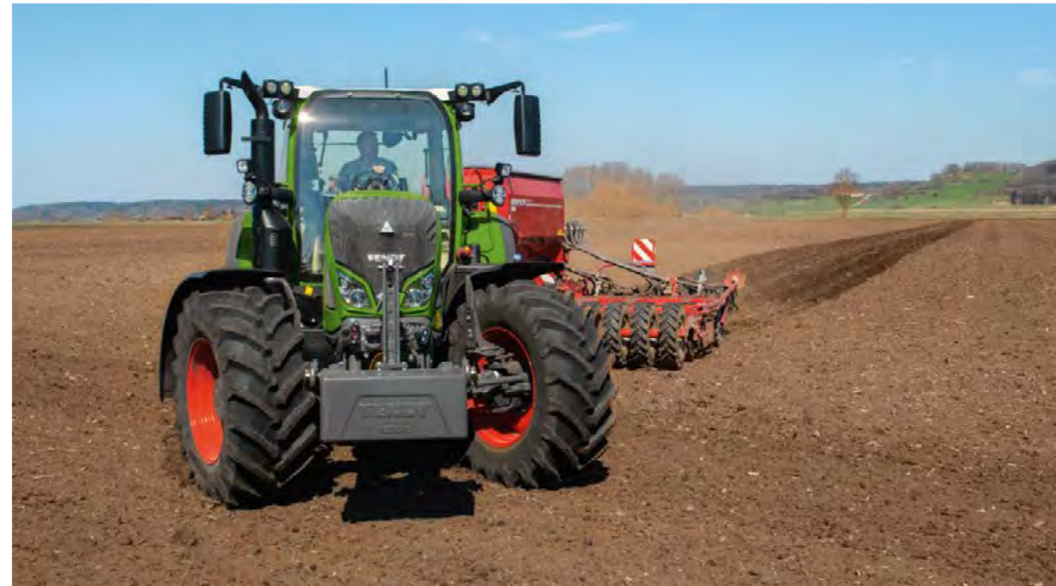
The high-end model – the Fendt 724 Vario – reaches its maximum torque of 1,072 Nm at just 1,500 rpm.
