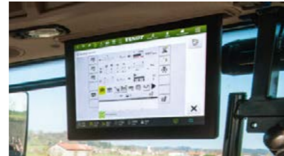
No need for an external ISOBUS terminal The additional 12" roof terminal offers you even more display space. You can show your ISOBUS attachment data on the roof terminal, for example, while the terminal on the armrest shows the lane guidance. External terminals are no longer needed.
