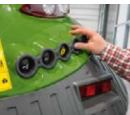
The rear power lift, PTO and one spool valve can be controlled from either rear fender.
