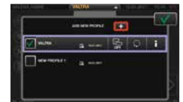
Profiles for operators and implements which can be easily changed from any screen menu. All the setting changes will be saved in the selected profile.
